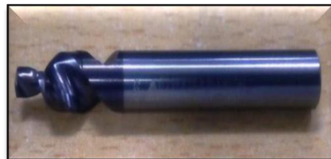
SC STEP DRILL D2.97XD6XFL20XOAL60
